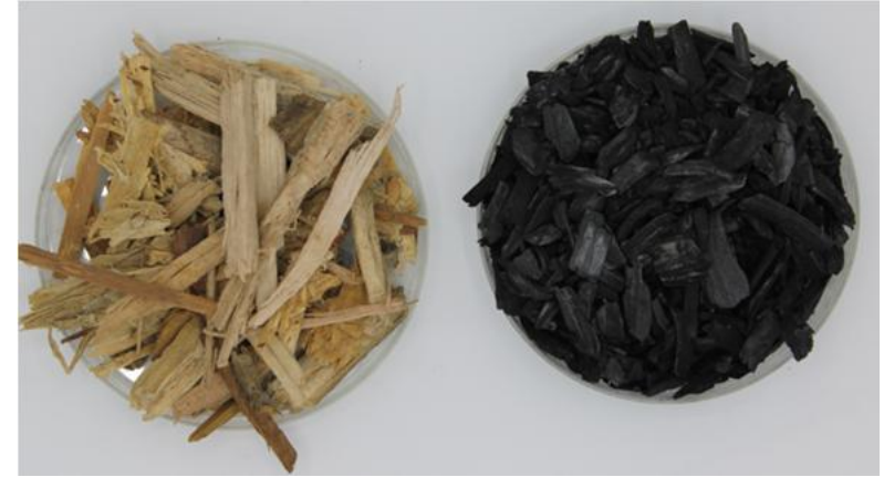
Fig 2. Woodchip before and after pyrolysis
